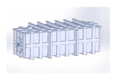
Aluminum chamber with reinforcement. Weight approx. 19,000 lbs. (8600 Kg) End blankoff flanges for initial testing.
