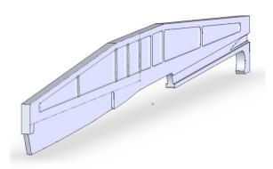
**Nov 7 (R6)** Added material at us end between clamping plates □deflection gets worse.
