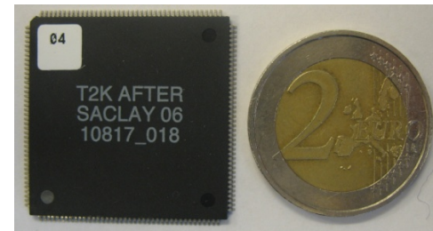
72 channel x 511 time buckets Switched capacitor array
