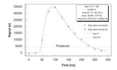
For first-order RC circuit, signal amplitudes sk can be deconvoluted from three measured values vk:
