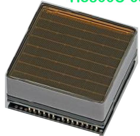
→ **H8500C-03**: typical gain (low),  $1.5 \times 10^{-6}$ , needs amplification X 100 to resolve SPE; noise could be an issue
