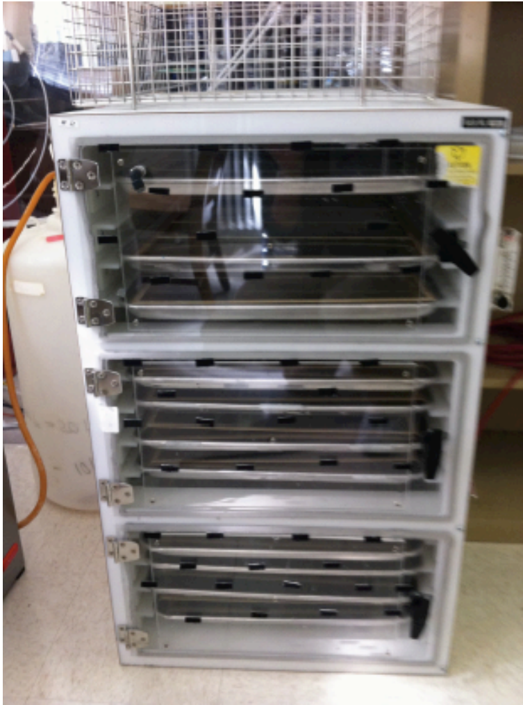
Dry N2 cabinet for frame storage
