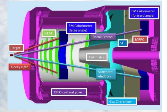
PID: E&M calorimeter for decay e<sup>-</sup>/e<sup>+</sup> additional gas Cerenkov for scattered e<sup>-</sup> MRPC-TOF for recoil proton
