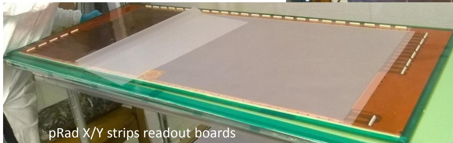
pRad X/Y strips readout boards
