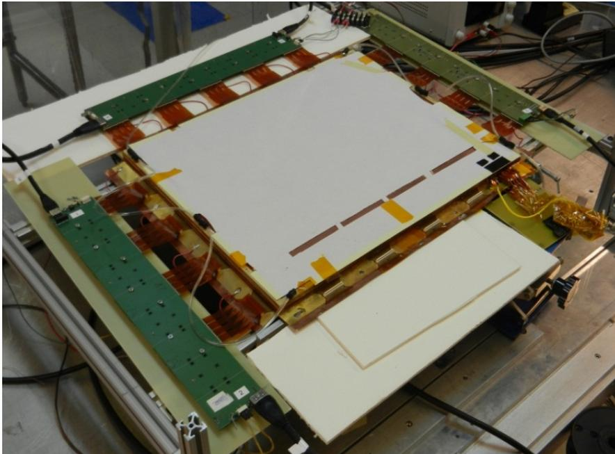
SBS prototype I: in bench tests with cosmics
