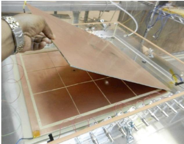
Loading the frame into the dry N2 box for testing at 4000 V
