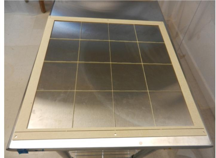
Flexible 2D readout board (CERN PCB workshop)
