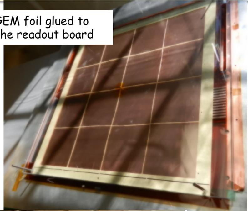
Four large dowel pins at the corners used to align the frames to within 100  $\mu\text{m}$
