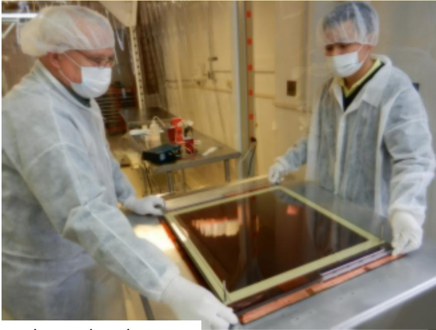
GEM foil glued to the readout board
