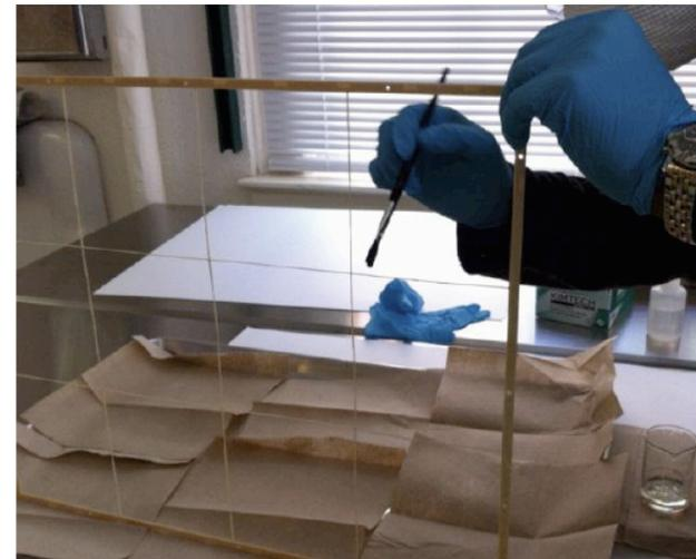
Machined surfaces sealed with a layer of polyurethane (Nuvovern LW) to prevent surface irregularities, residual fibers or sharp edges in the active area of the chamber
