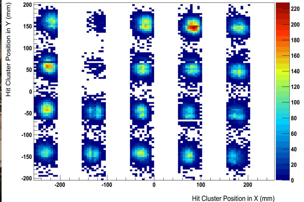
Data from the SBS prototype II - a powerful  $^{90}\text{Sr}$  source was used for this test. One sector (out of 20 sectors) shows lower efficiency
