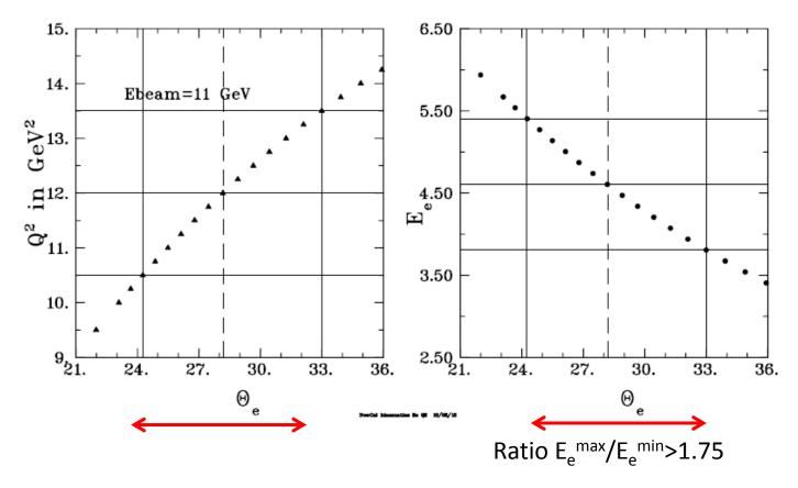
2. Wide distribution of constant  $Q^2$  profile on face of Ecal **Left**, number of events on SBS side, **Right**,  $Q^2$  on Ecal side. Boxes proposed coverage by new Ecal. Follow the green area, which is 11.5 to 13.5 GeV<sup>2</sup>. Electron energy is then 5.5 to 3.3 GeV. Figures from Mark Jones, SIMC simulation.
