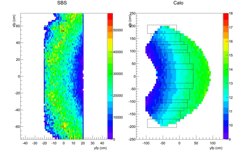
2. continued, same as previous, but with acceptance cut on ECal enforced. The detector configuration shown contain 304 11.2x11.2 cm<sup>2</sup> detector bars. The distance to the back of Ecal is 6.35 m.
