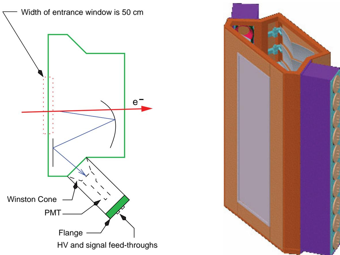
Figure 14: Cross sectional view and schematic of the Cherenkov counter of the BigBite Spectrometer. Cherenkov light is reflected from 20 spherical mirrors back to two flat mirrors and then directly or indirectly through Winston cones on the phototubes.
