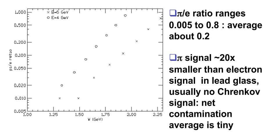
Pion asymmetry will be measured with very high precision with both the scalar and FADC electronics
