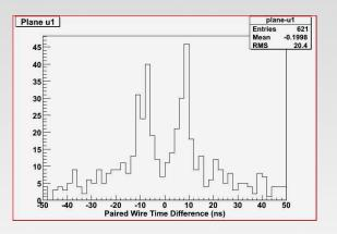
Second signal appears to be about  $7ns\pm 3ns$  after first signal Removal reduces hits by 12% in chamber 1 and 5% in others
