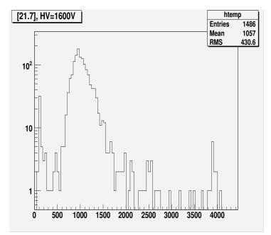
ADC amplitude peak around channel 1000 with 1600V.
