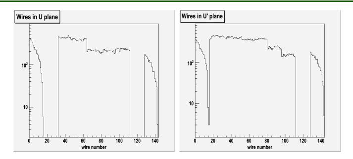
• The empty region in the plot corresponds to the wires with missing amplifier cards
