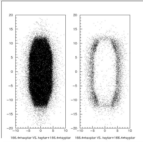
Aperture defining collimators in HMS/SOS not completely effective at stopping hadrons (protons, pions)
