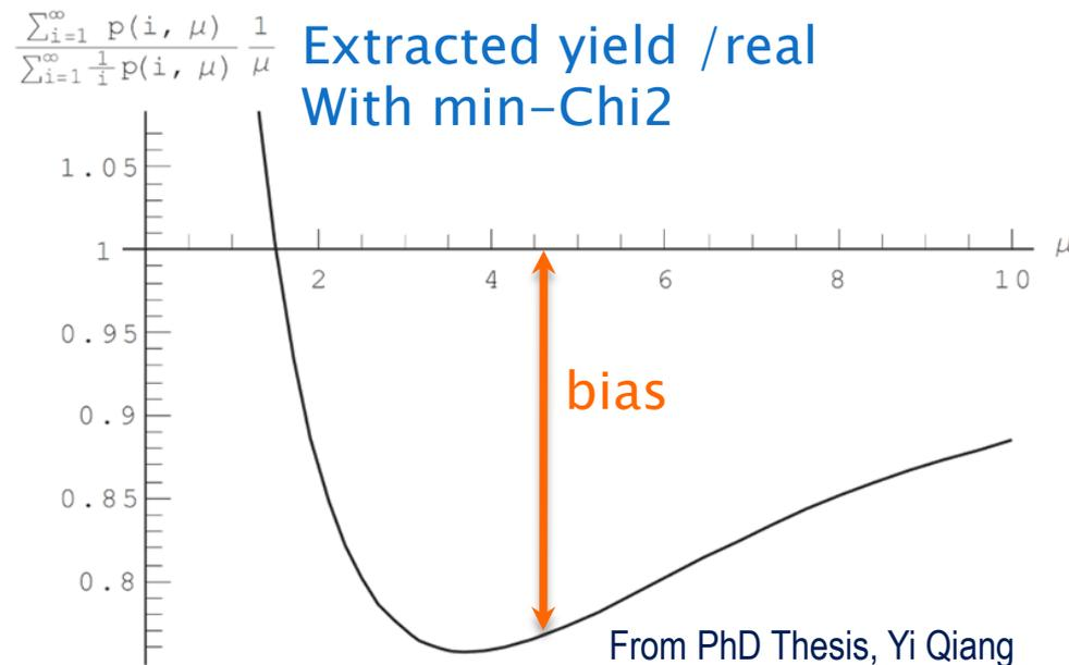
The ratio of weighted average to true value  $\mu$  as a function of  $\mu$ .
