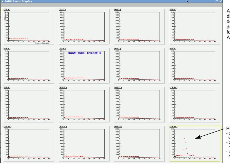
A simple event display was developed as a diagnostic tool for JLab Flash ADC readout
