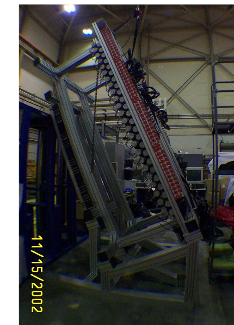
Figure 6: Photograph of the completed charged particle detector package.
