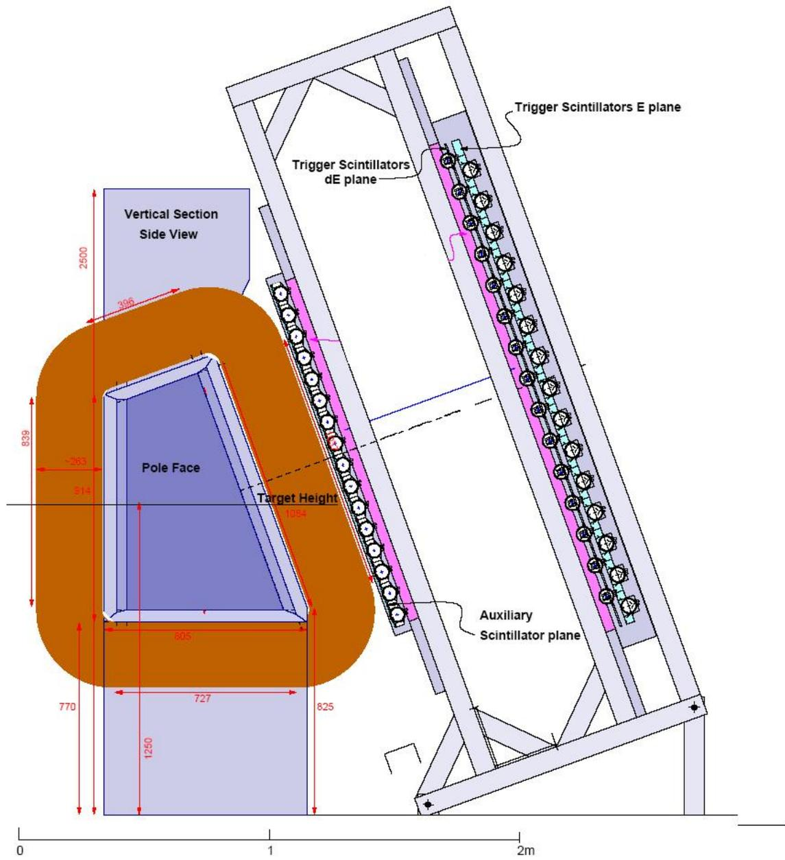
Figure 3: Side view of BigBite with initial detector package
