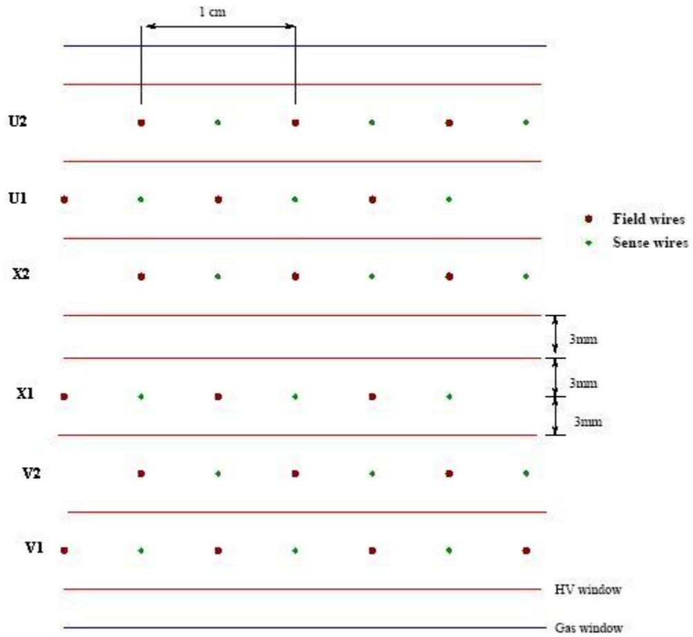
Figure 4: BigBite wire chamber layout.
