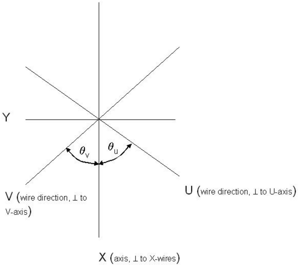
Figure 12: illustration of coordinate system and angles used in rotation matrices
