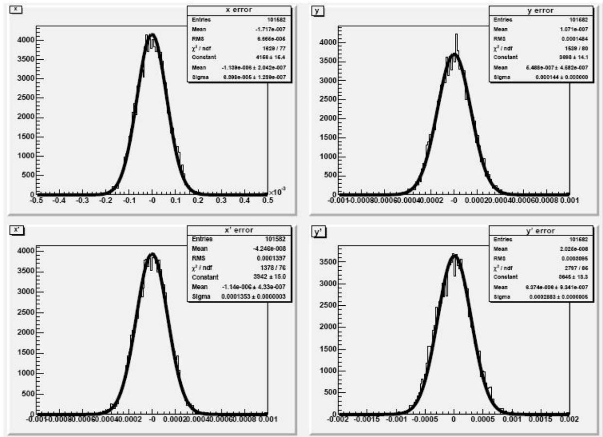
Figure 13: Histogram of errors in  $(x, y, \theta, \phi)$  for reconstructed tracks
