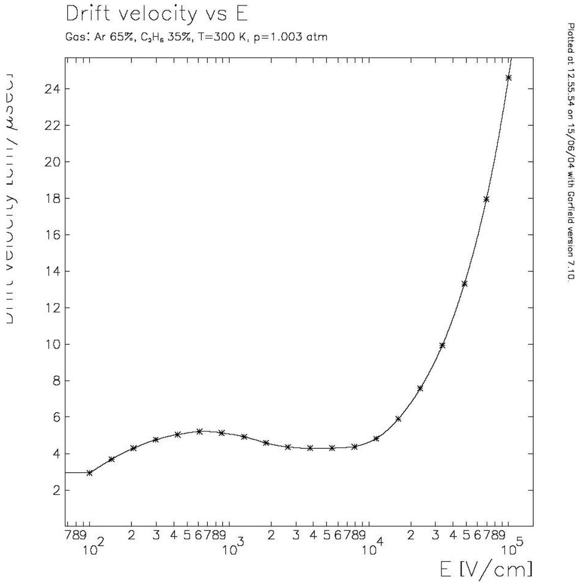
Figure 5: Drift profile for BigBite wirechamber gas mixture calculated by GARFIELD's interface to the Magboltz program
