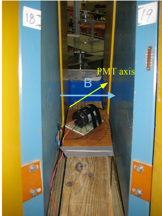
Figure 5: The fine mesh PMT module H6614 in the gap of the BigBite magnet in Hall A. The blue arrow indicates the direction of the magnetic field and the yellow arrow indicates the direction of the PMT axis. The angle between the two directions is labeled \theta in this report.
