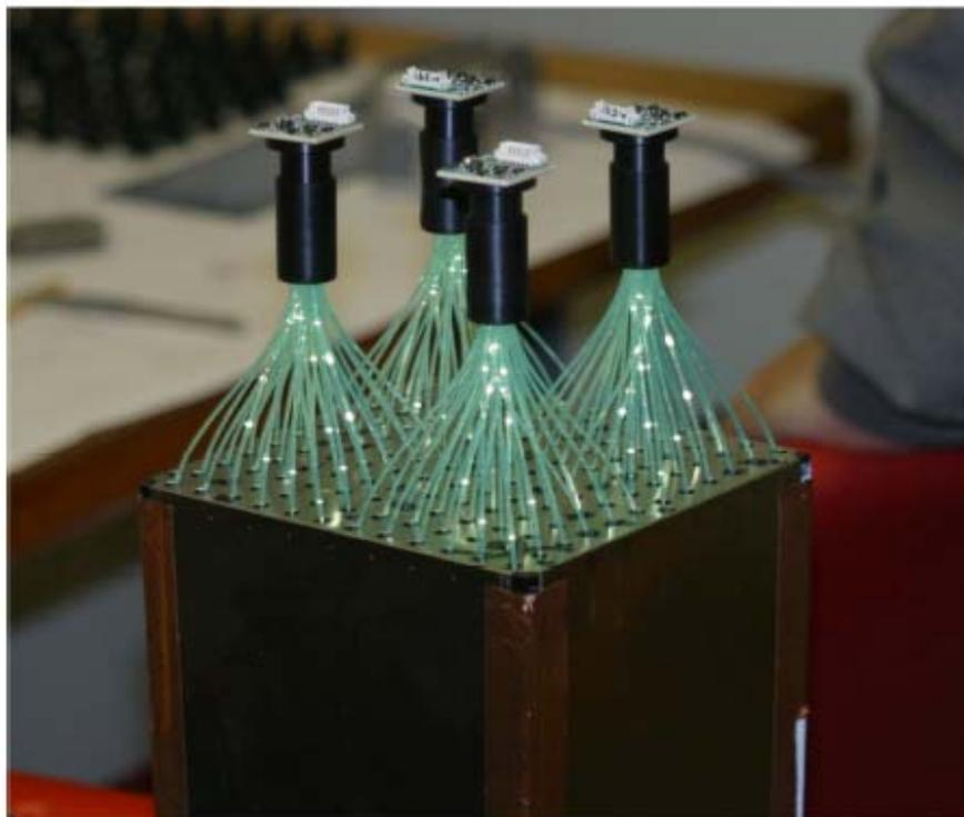
Figure 1 - EMCAL module with optical and electronic readout
