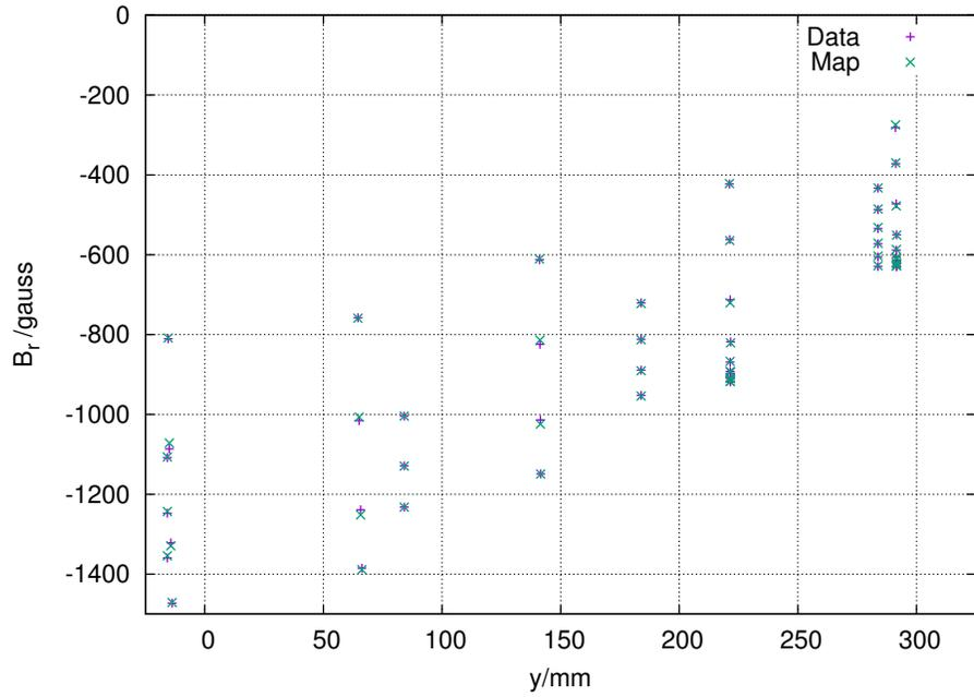
Figure 3: Measurement result of  $B_r$  (Data) and the calibrated value from the field map (Map).
