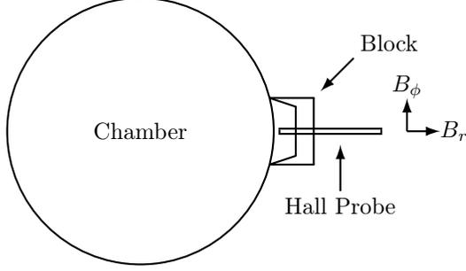
Figure 1: Sketch of the experiment setup. The azimuth direction Hall probe is not shown in this figure.
