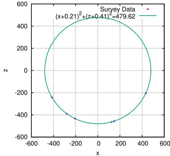
Figure 2: This figure shows that all survey points fits the same cylindrical surface after calibration.
