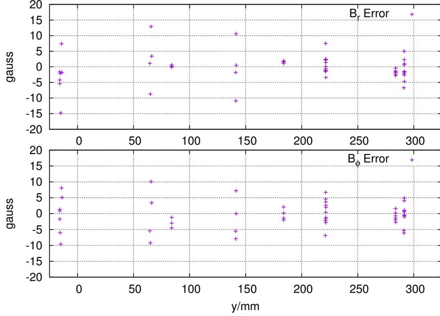
Figure 5: The distribution of the differences between the measured field and the field map.
