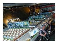
Radiator 15 mm thick Liquid Freon  $(C_6F_{14}, n=1.28)$
