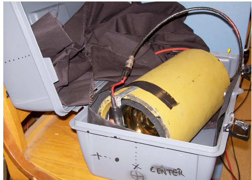
PMT wrapped in blackout paper, placed in iron shield
