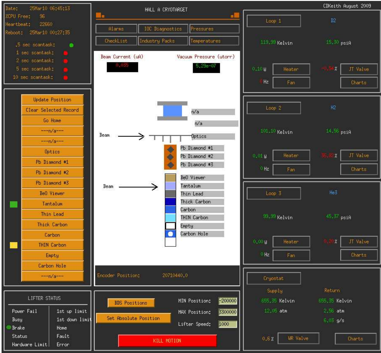
FIGURE 2. Control GUI for the Lead target. The C-REX target is similar. And of course, this is just a rough draft copied from PREX-I.
