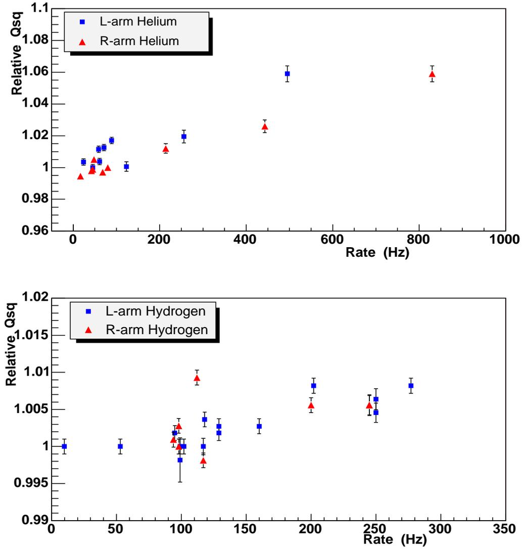
FIG. 1: Effect of rate on  $Q^2$  (relative units). Distortions for  $^4\text{He}$  occur in spite of the cut that demanded only one good track because of the quasielastic peak, and we used data only below 100 kHz. The Hydrogen result shown in this plot did not require a 1-track cut, although it was done for the final result in fig 2. In contrast to  $^4\text{He}$ , the 1-track cut makes the Hydrogen result constant, and all data are used. See text for why.
