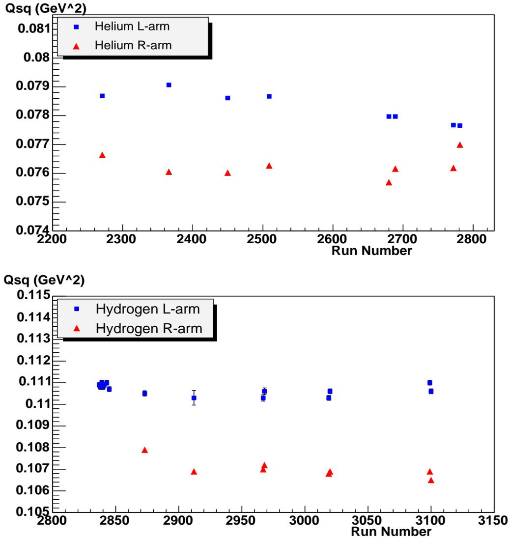
FIG. 2:  $Q^2$  versus run number during HAPPEX 2005 for  $^4\text{He}$  (top) and Hydrogen (bottom). These have been ADC weighted. Standard cuts are: 1) One track; 2) Track deposits energy in HAPPEX detector; 3) Track within collimator acceptance.
