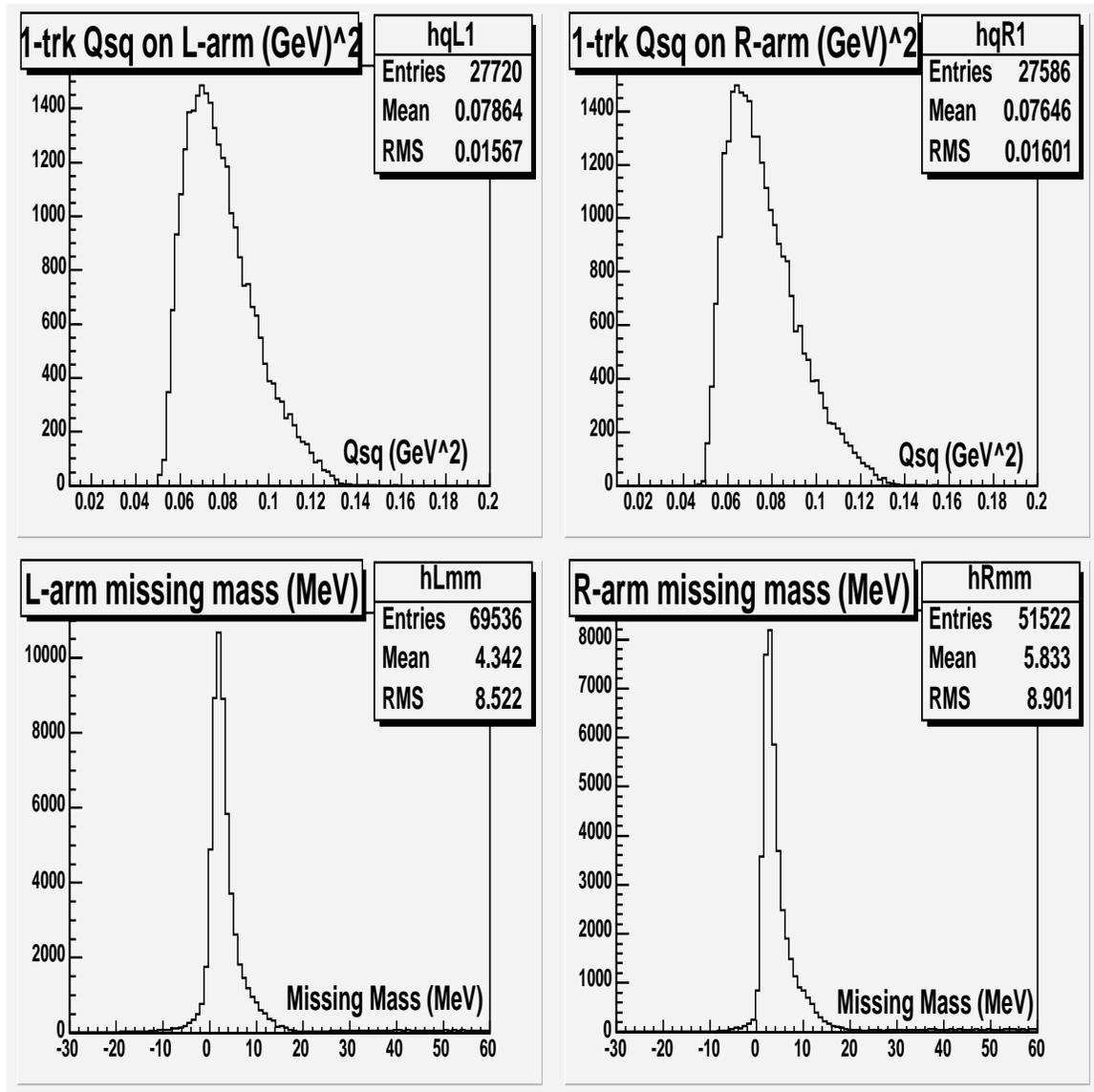
FIG. 3: Typical Helium  $Q^2$  on Left and Right HRS (top row) and missing mass (bottom row). Not weighted by ADC. The missing mass peaks a few MeV from zero, consistent with our systematics – also for Hydrogen.
