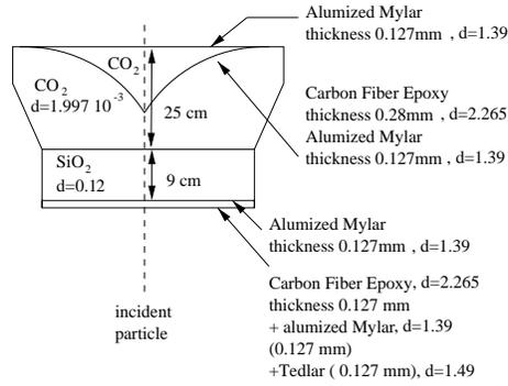
Fig. 4: cross section of the aerogel Cerenkov. The densities ( $d$ ) are in  $\text{g}/\text{cm}^3$ .
