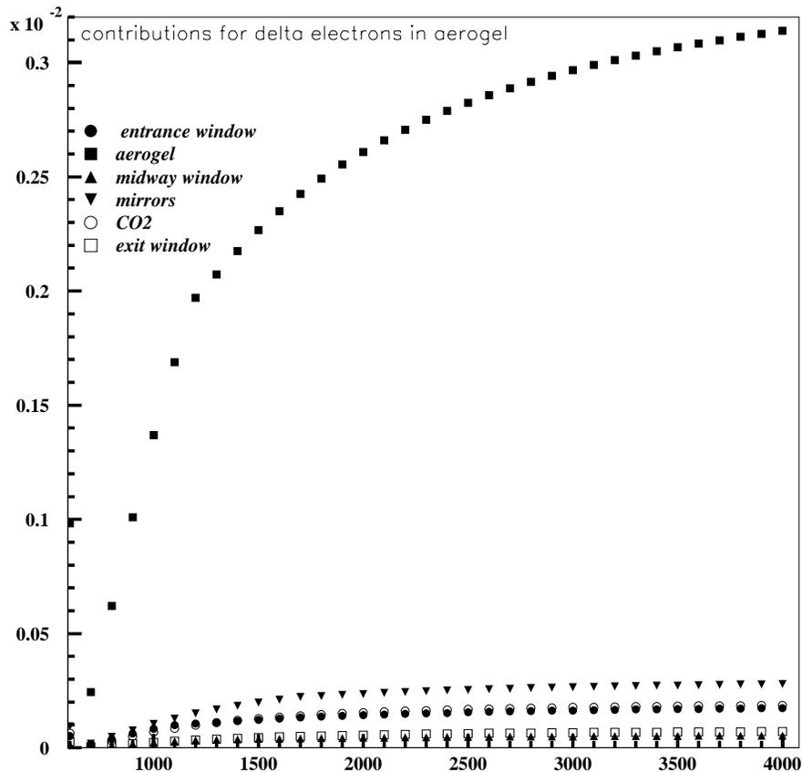
Fig. 7: detail of the different part contributions for the aerogel Cerenkov
