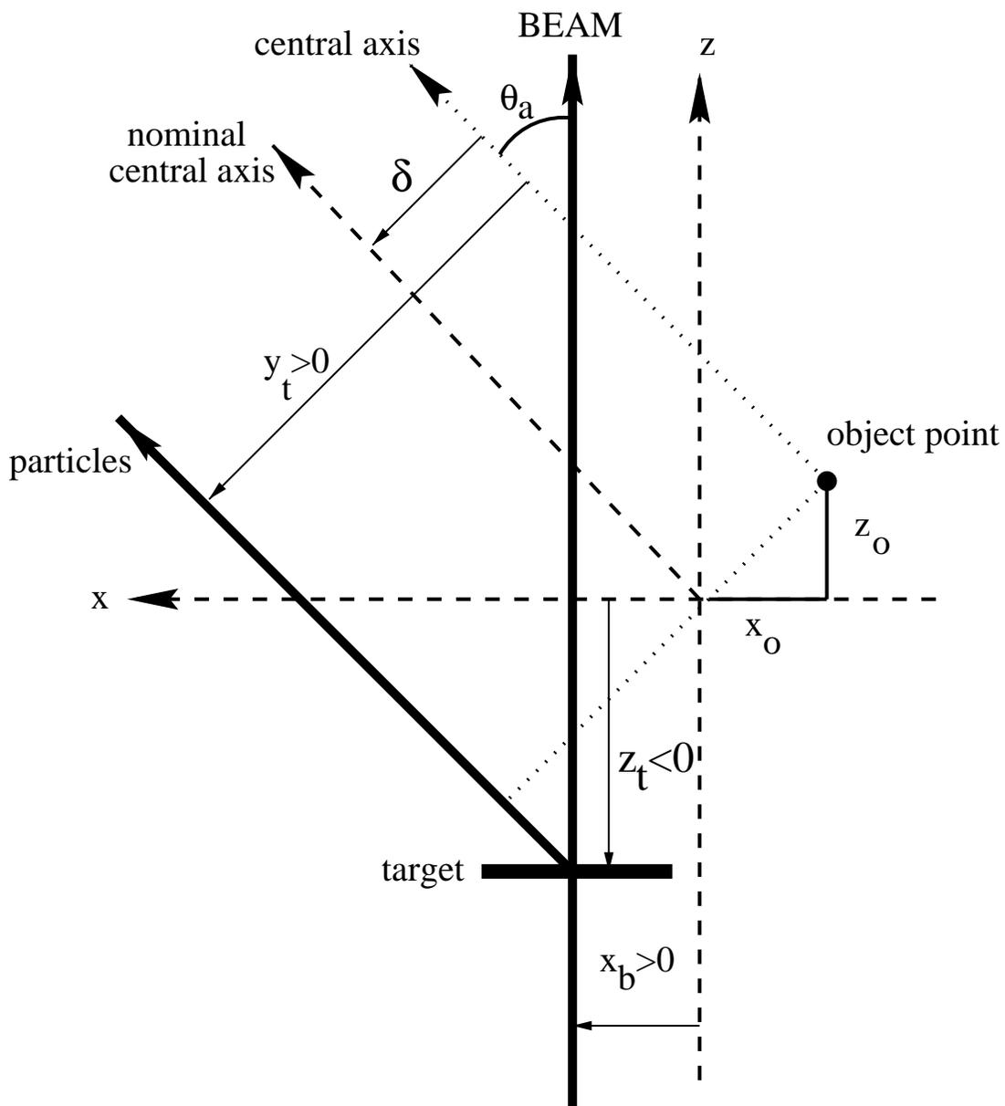
Figure 1: Geometry for determining the pointing offset of a spectrometer.
