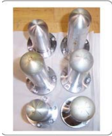
Figure 1: Cryotarget cells: machined cylindrical ‘cigar-tube’ style.
