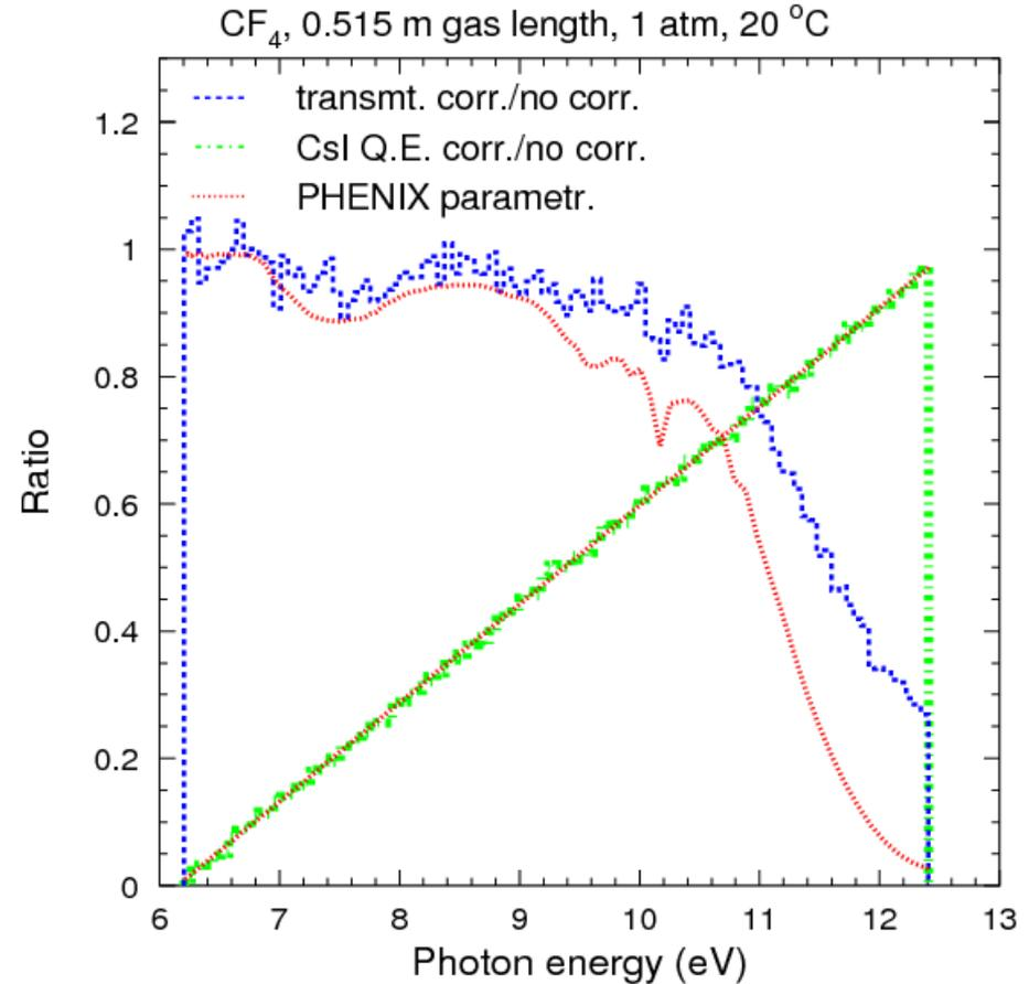
The photocathode Q.E. is taken into account as an energy-dependent correction
