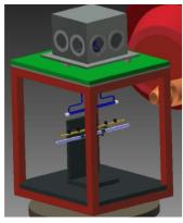
Above, and above right: Rendering of multiple-pumping-chamber target for A1n experiment that will run prior to Super Bigbite at 30µA.
