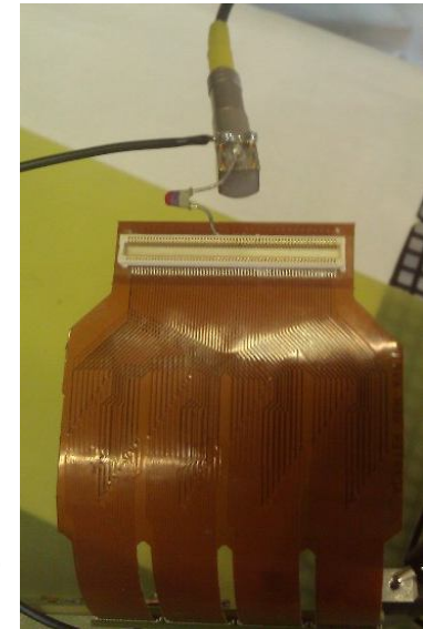
Signal through ~3 pF capacitor soldered on 4 channels
