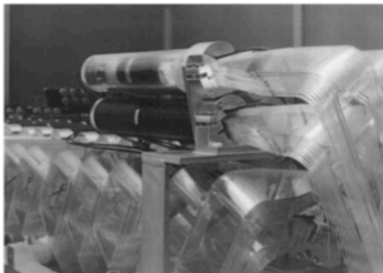
Coupling of scintillators to PMTs
