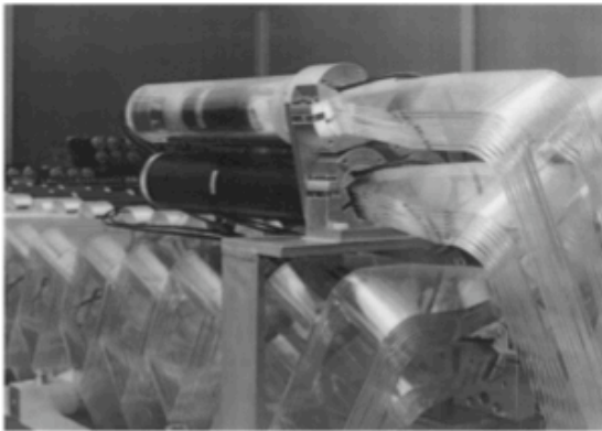
Coupling of scintillators to PMTs
