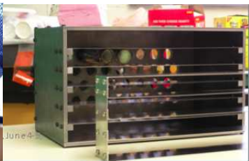
(c) prototype box with steel bars and \mu -metal shelf
