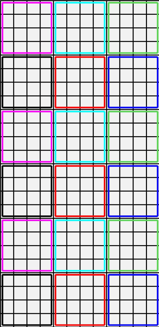
Triggering scheme being investigated by Monte Carlo based on dividing modules into groups of 4X4
