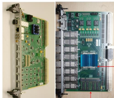
FPGA based digitizer MPD(INFN, Paolo) Subsystem processor (JLab customized electronics)
