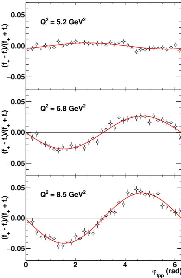
$$f^+ - f^- \equiv \frac{\pi}{\Delta\varphi} \left[ \frac{N^+(\varphi)}{N_0^+} - \frac{N^-(\varphi)}{N_0^-} \right] \\ = \bar{A}_y [P_{y,tr}^{FPP} \cos \varphi - P_{x,tr}^{FPP} \sin \varphi] \times [1 + \mu_0(\varphi)] \quad (24)$$
