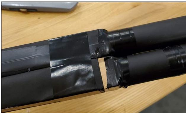
Figure 4: Scintillator covering.
