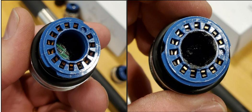
Figure 5: PMT base as it comes from the factory. (Left) PMT base with RTV sealant in the opening. (Right)
