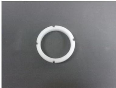
6) Attach the "base collar" to the PMT base using a plastic set screw. An o-ring placed on the PMT base seals any possible light leak from the gap between the "base collar" and the PMT base. The nylon washer goes around the PMT.
