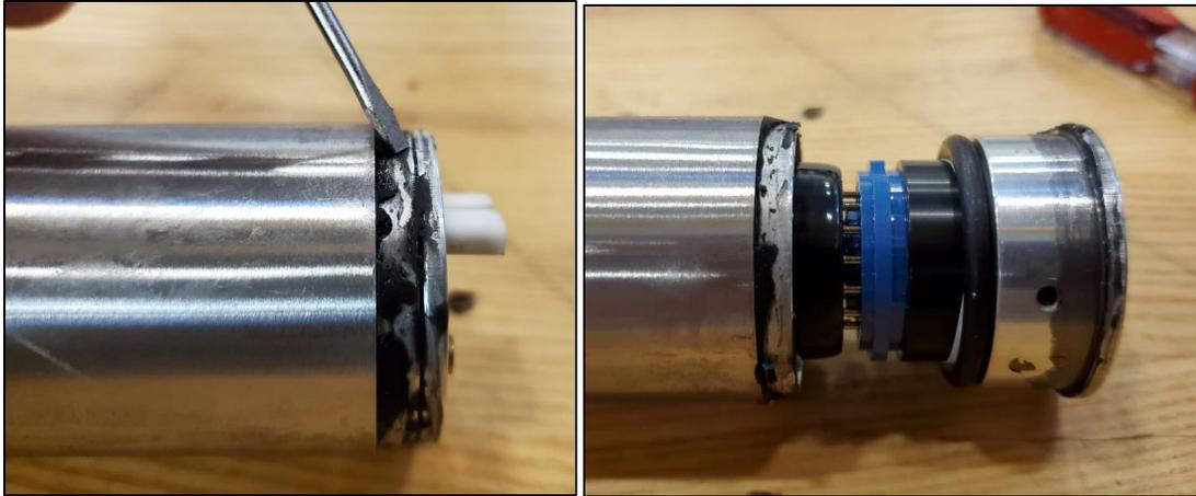
Figure 2: Two pictures of the PMT assembly and the RTV sealant around the PMT base collar and the mu-metal and inner aluminum pipe. This RTV sealant makes removal of the mu-metal and the PMT base and base collar very difficult.
