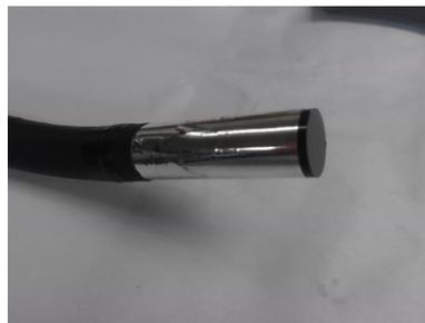
3) Prepare one gas inlet, made of stainless steel tube  $3/32$ " of external diameter and 0.5" long (not longer than this, so the heat shrink can still be inserted).
