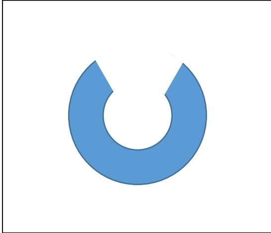
*Figure 10: Drawing of the "horseshoe" shape recommended for dealing with the stuck nylon washer issue.*
