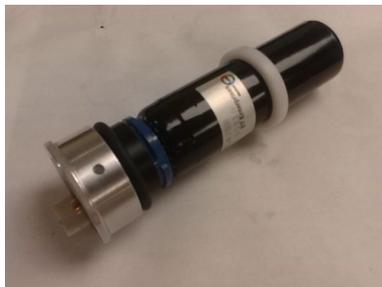
7) Attach the part from item 4 to the light guide using the “clamps”. The PMT setup is then placed in the “Al pipe”, making sure the PMT is touching the light guide. We could think about a spring based device to make sure the PMT is pressing against the light guide, so the PMT is always in contact with the light guide. What is the best alignment for the gas inlet relative to the bar?
