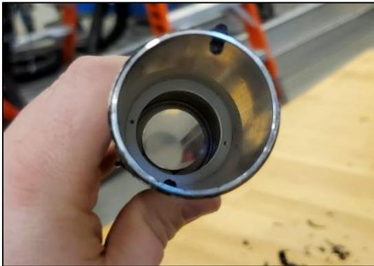
Figure 3: A picture of the nylon washer in the aluminum pipe.
