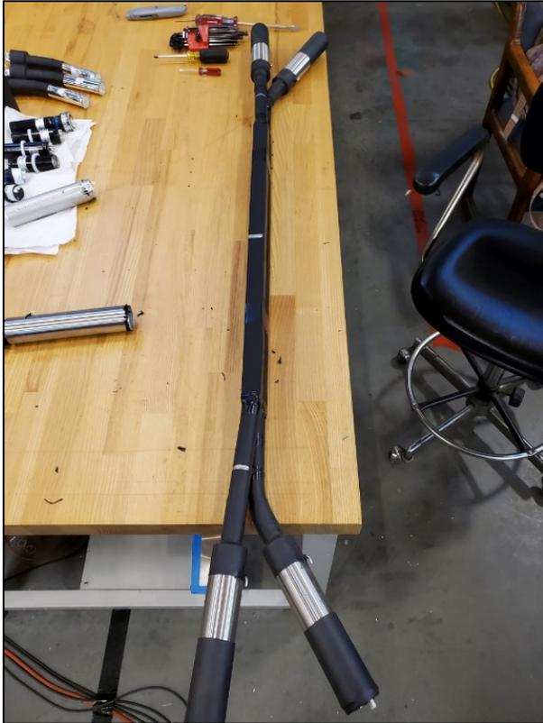
*Figure 1: Photo of a two scintillator assembly showing the straight versus curved light guides. The extra length to the light guides is necessary for the PMT assemblies to both clear each other and to clear the Big Bite frame.*
