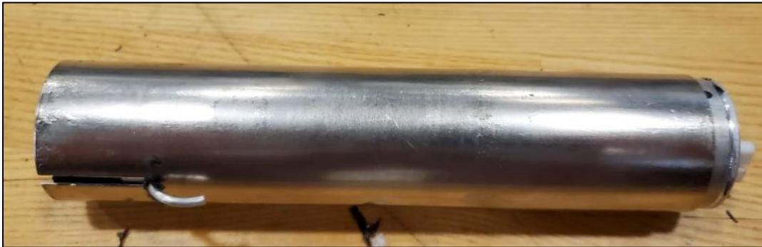
Figure 8: PMT assembly with mu-metal shield.
