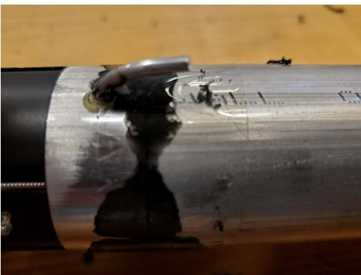
Figure 7: Connection point between the aluminum pipe and the light guide clamp collar. The small tube is the gas inlet port.
