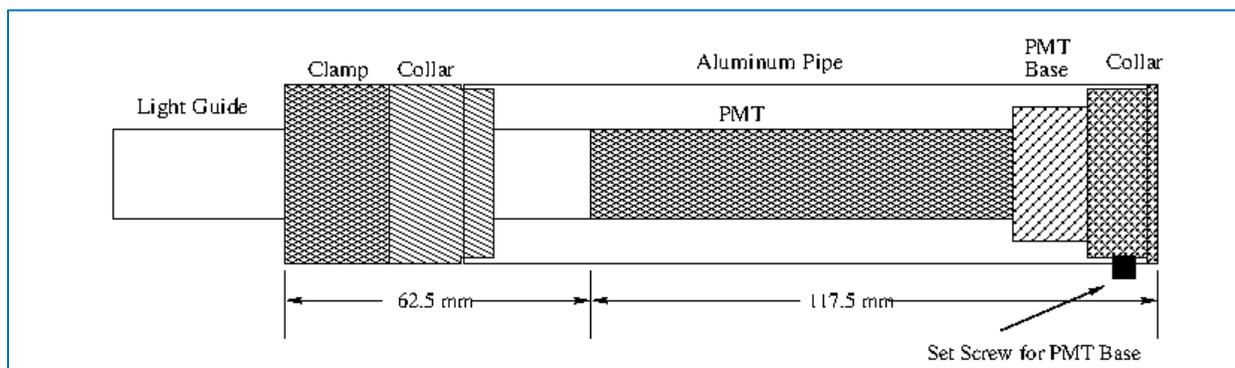
Figure 11: Schematic of the PMT assembly without mu-shield.
