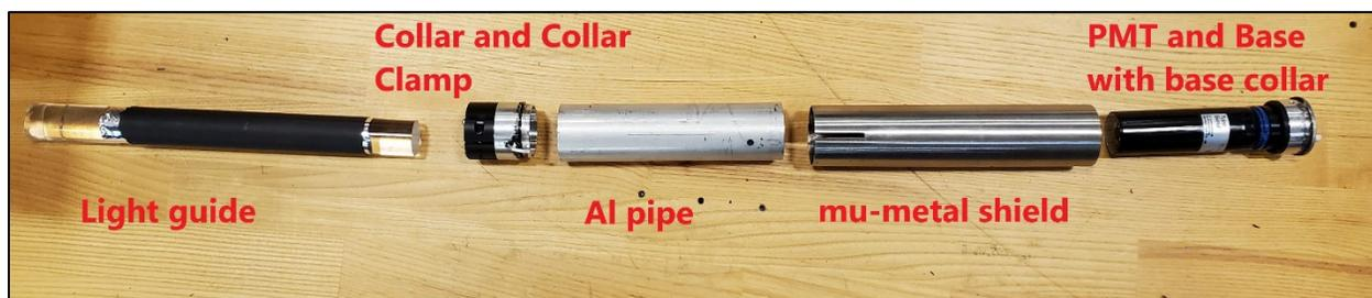
Figure 12: Partially disassembled assembly from the light guide to the PMT base.
