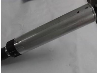
8) Insert the mu-metal, with the gas inlet going through the slot.
