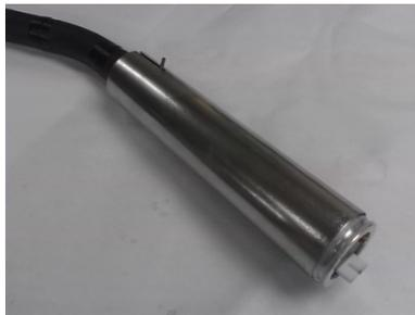
9) Use heat shrink tube for sealing the region of the “clamp collar”/light guide, and also the region of the PMT base.
