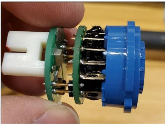
Figure 6: RTV sealant penetration into the wiring area of the PMT base.
