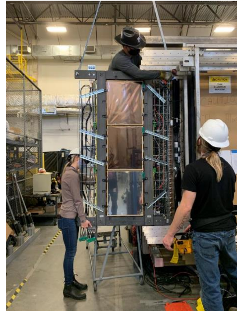
Installation of two INFN GEM layers in Bigbite before moving to the Hall February 2021
