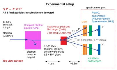
Trigger: GEMs, hodoscopes, calorimeters (all 3 particles)
