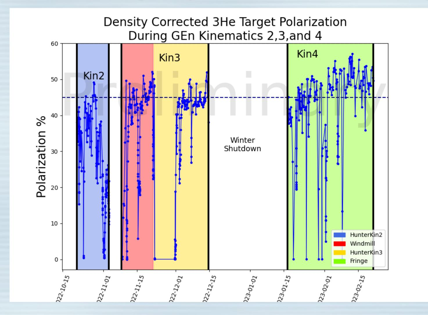
For reference – with the 60cm target chamber, a polarization of 45% and 45 $\mu$ A of beam, the figure-of-merit compared to A1n (assumed to be 50% with 30 $\mu$ A beam) is x 1.82 higher.
