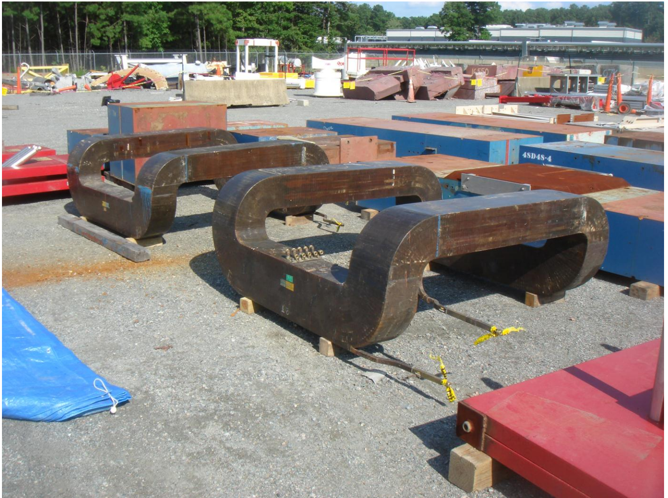
Figure 1: Saddle coils from the 48D48 magnet at JLab
