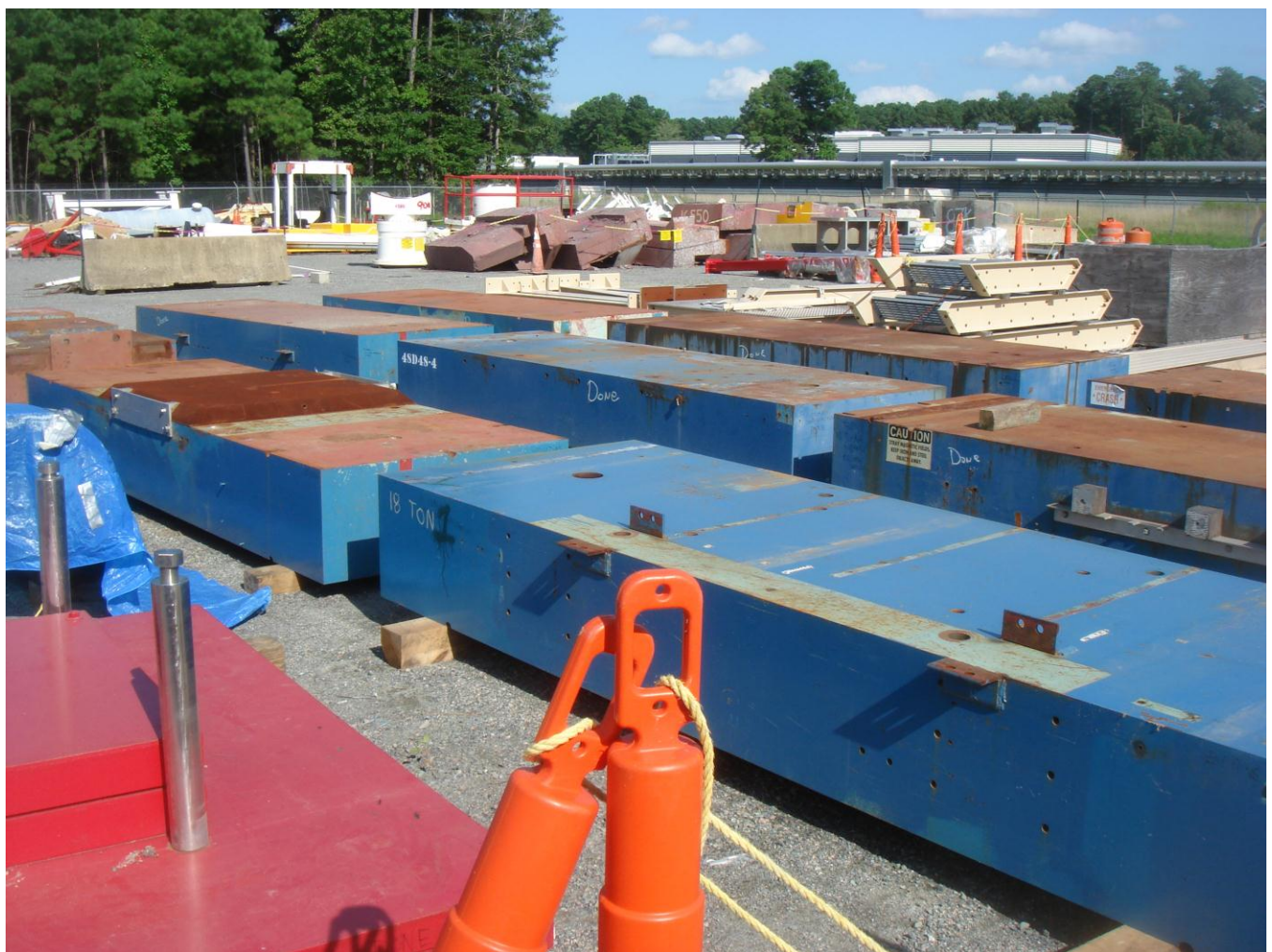
Figure 2: Yoke pieces for the 48D48 magnet at JLab
