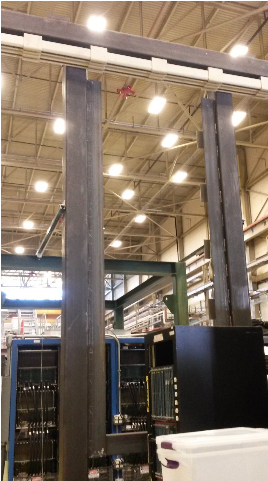
Figure 5: Coordinate Detector: A photo showing the large vertical frame which will hold the two planes of modules.
