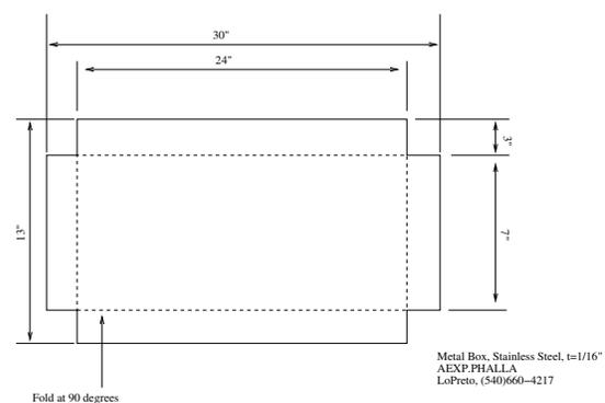
FIG. 3: Metal Container Bottom
