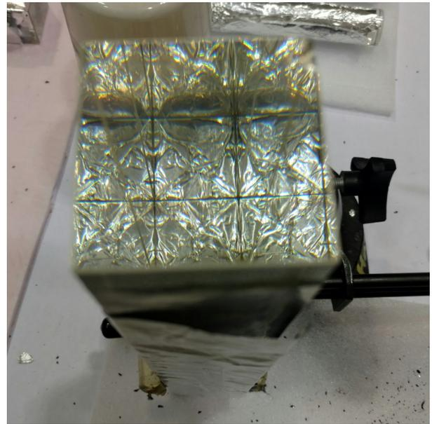
FIG. 6: Eccobond F202 Bipax on lead-glass after baking at 340 °C and scraping with razor blade.
