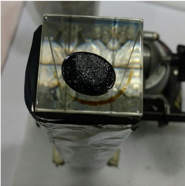
FIG. 5: Eccobond F202 Bipax on lead-glass after baking at 340 °C.
