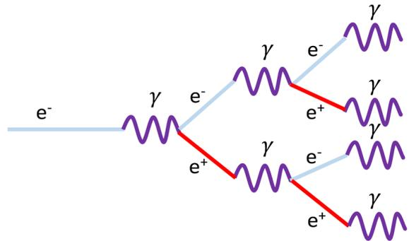
FIG. 1: Particle shower produced by alternating Bremsstrahlung radiation and pair-production.
