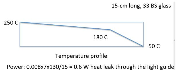
FIG. 2: Temperature profile for lead-glass in new high-temp EM calorimeter. Taken from Reference 2.
