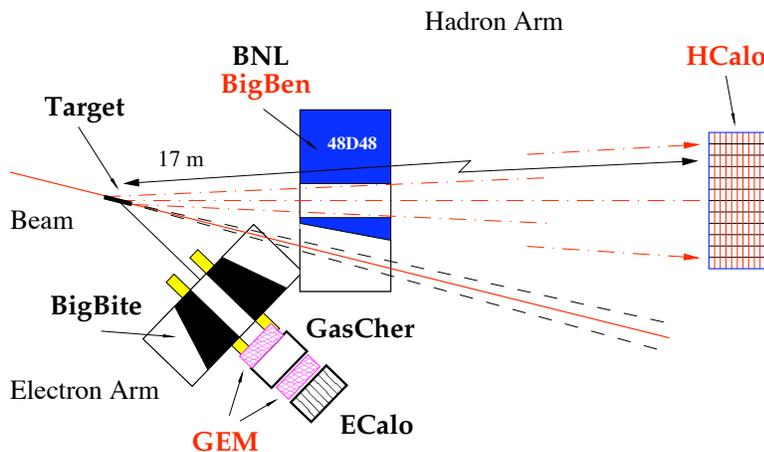
Figure 2: Shown is a schematic representation of the setup that will be used for both the GEN (E12-09-016) and the GMn experiments (E12-09-019). The target will be polarized  $^3\text{He}$  for GEN and deuterium for the GMn experiment, most other components are identical.
