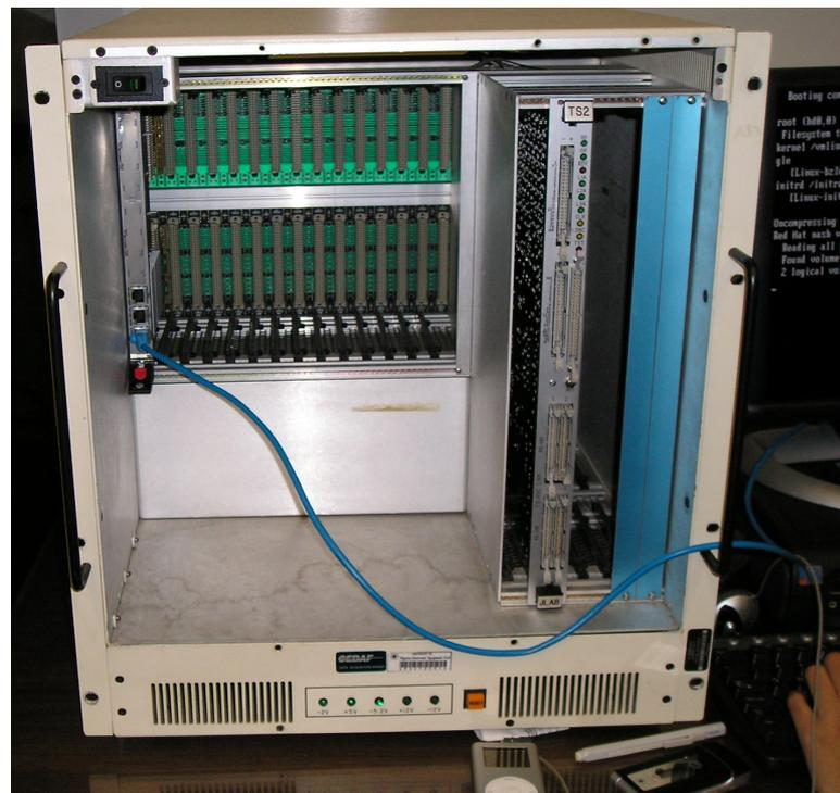
Rutgers DAQ: VME6100 and trigger supervisor, before v1495s installed
