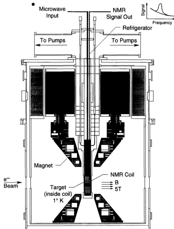
Fig. 1. Schematic of the E143 polarized target.
