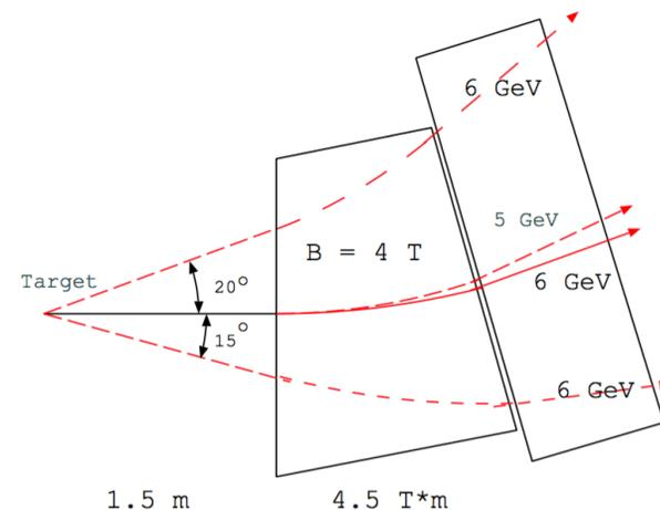
Figure 4. A side view of the Super BigBite.
