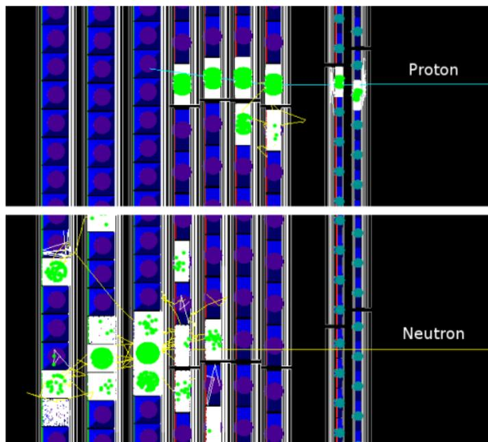
Side view of ND depicting the ideal scenario of charge ID. The recoiling nucleons have an energy of 1.3 GeV prior to entering the detector.
