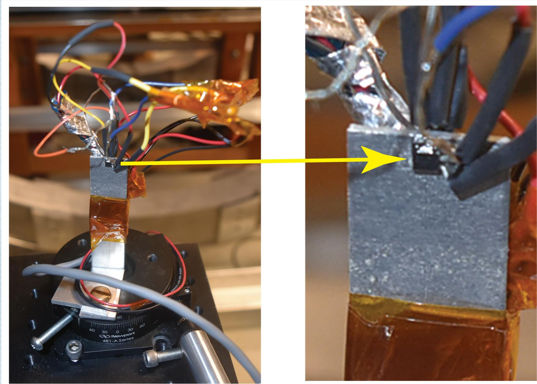
Shown is the Hall Probe mounted on a precision rotation stage for sensitivity study.
