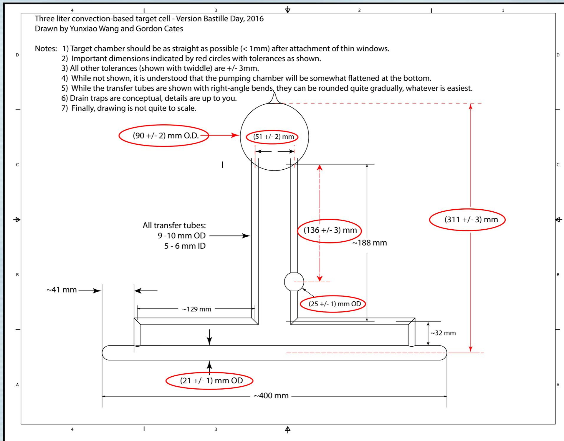
Note that the pumping chamber extends from roughly 22.1cm to 31.1 cm above the center of the target chamber.
