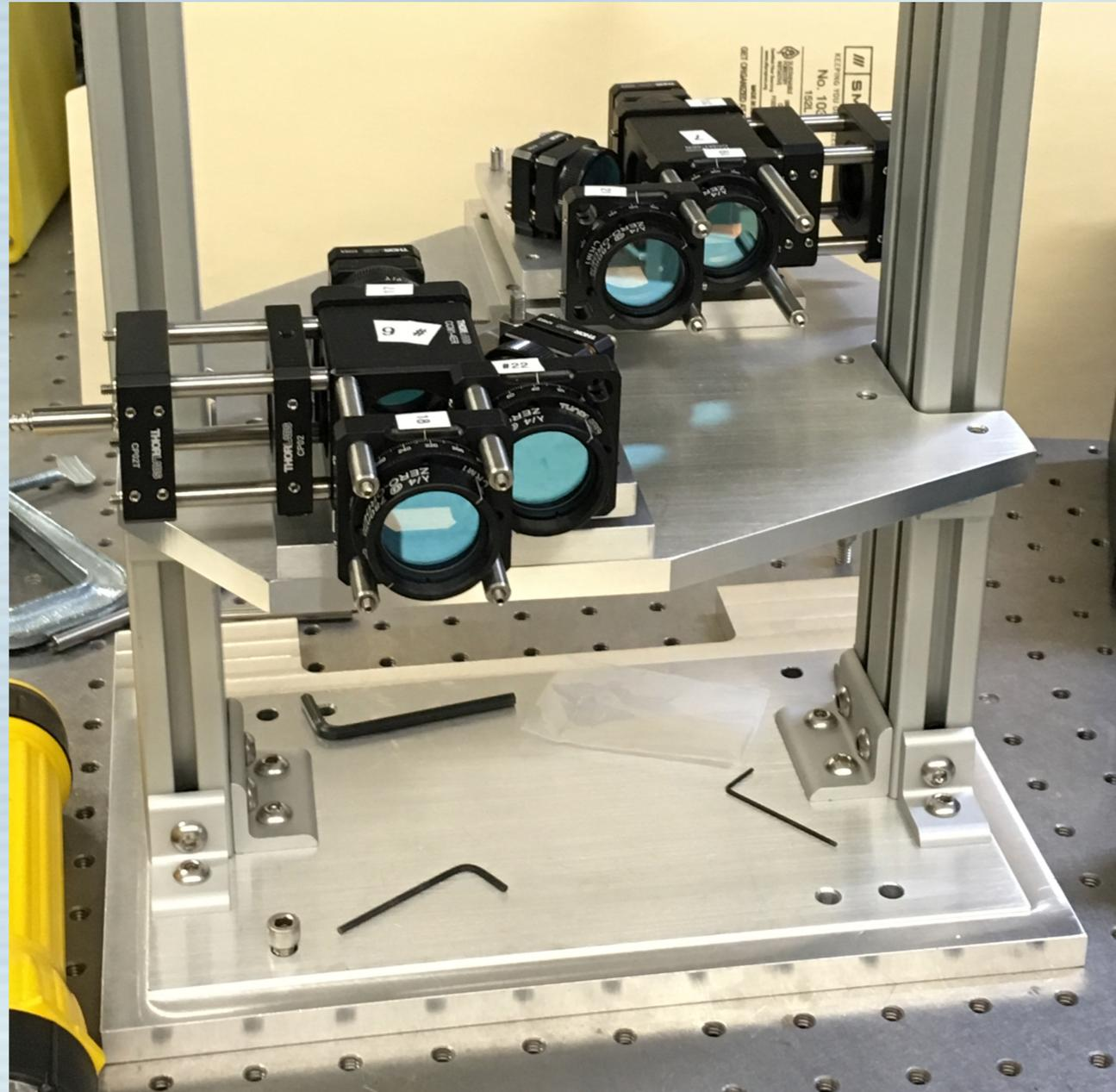
Two out of four of the optics modules for SBS. The next two modules will “hang” from a second platform stacked above the platform shown.
